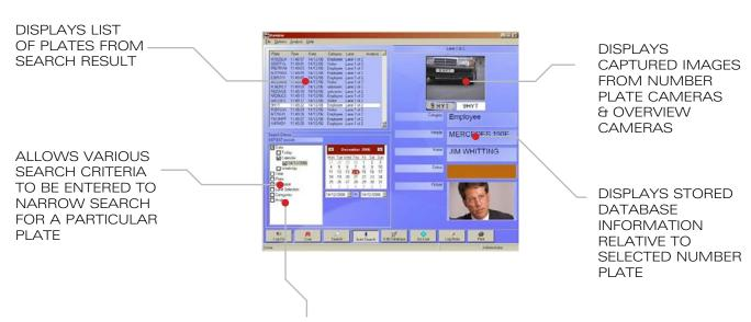
ANALSYIS OF RECORDED DATA CAN BE CARRIED OUT SUCH AS FREQUENCY OF ENTRIES, CAR PARK OVERSTAY, SPEED BETWEEN POINTS
